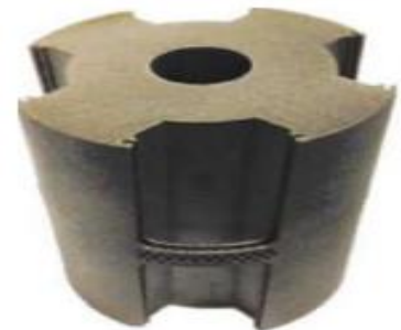
Figure 4: (a) 3D-printed hairpin distributed windings for E-traction motors and (b) 3D-printed skewed rotor (Ahmed, Mohamed, and Peter, 2022).
